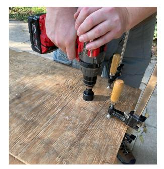
Using hole saw to cut acrylic sheets through pre-drilled holes (jig).
